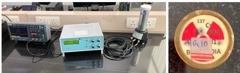
Figure 1: Experimental setup (left) and ^{137}\text{Cs} source (right)
